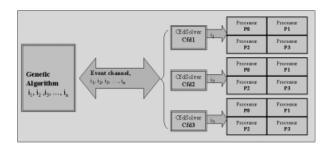
Fig. 4. Interaction between the genetic algorithm and the CFD solvers.
