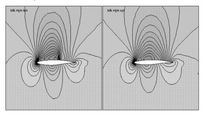
Fig. 2. Wing shape optimisation: induced drag reduction in high-speed cruise configuration
