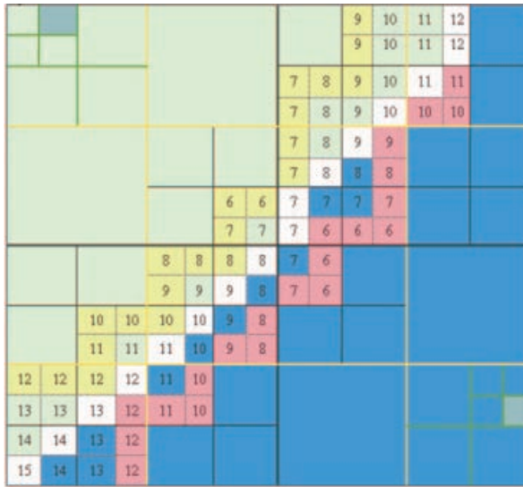
Fig. 5. The hierarchical implementation for Voronoi diagrams using the mixed distance calculation based routine (Total pixels for distance transform 16+40+84=140 , but total pixel will be 256 using non hierarchical methods)
