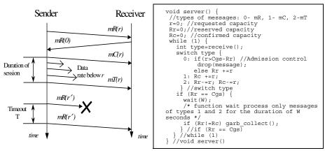
Fig. 2. Setup and tear down of reservations.
