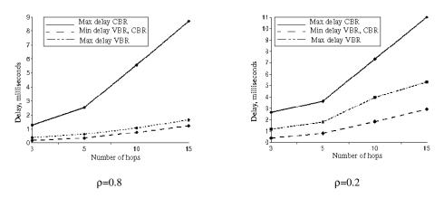
Fig. 13. Min and max delays for GS flow for VBR and CBR.
