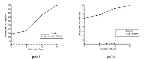
Fig. 12. End-to-end jitter of the monitored GS flow for the VBR case.
