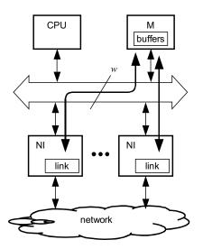
Fig. 1. First Generation Store-and-Forward IP Router
