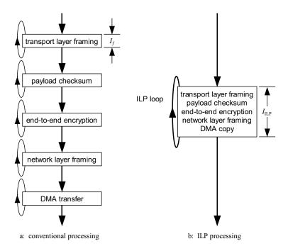
Fig. 4. Conventional and ILP Processing for TCP/IP
