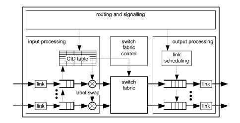
Fig. 2. Connection-Oriented Fast Packet Switch
