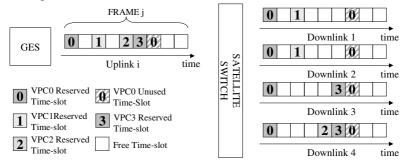
Fig. 5. Uplink and downlink reserved capacity
