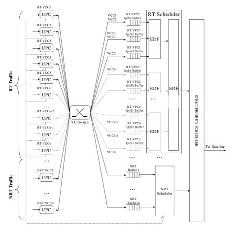
Fig. 3. Proposed gateway architecture
