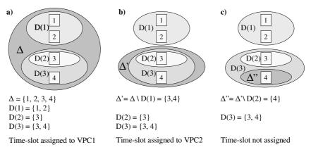
Fig. 6. Downlink sets for the stolen slot procedure
