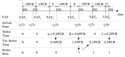
Fig. 4. Example of the stolen slot algorithm
