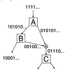
We do not want the graph spreading out continuously. On the contrary, some pulse paths are collected in adders. In particular, a final adder gives just one output of the graph.
