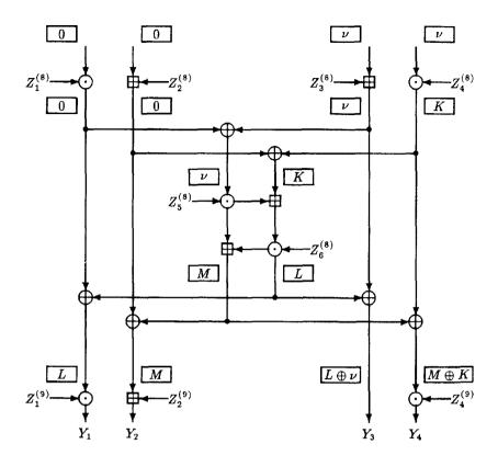
Fig. 2. XOR propagation of  $X' = (0, \nu, 0, \nu)$  through the last round of IDEA for keys with only nonzero bits on positions 26-40, 72-83 and 99-122. The XORs are indicated in boxes.
