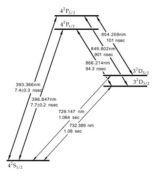
Fig. 3. The lowest energy levels of  ${}^{40}Ca^+$  ions, with transition wavelengths and lifetimes listed.
