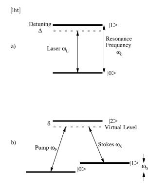
Fig. 2. A schematic illustration of (a) single laser and (b) Raman qubit addressing and control techniques.
