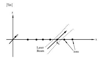
Fig. 1. A schematic illustration of an idealized laser-ion interaction system;  $\mathbf{k}_L$  is the wavevector of the single addressing laser.
