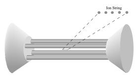
Fig. 4. Side view diagram of the linear RF trap used to confine  $Ca^+$  ions in these experiments. The endcap separation is 10 mm and the gap between the RF rods is 1.7 mm.
