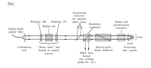
Fig. 6. Illustration of the laser beam control optics system.
