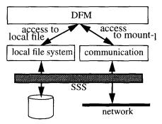
Fig. 12. The Distributed File system Manager switches user accesses either to local file system or to a server
