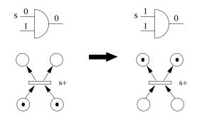
Fig. 4. Synchronized signal switch and transition firing
