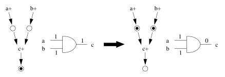
Fig.7. Stable AND gate becoming excited by backward switching
