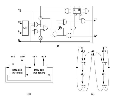
Fig. 11. (a) DME cell; (b) Two user DME ring; (c) Petri net specification
