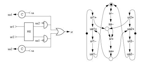
Fig. 1. A circuit and its Petri net specification
