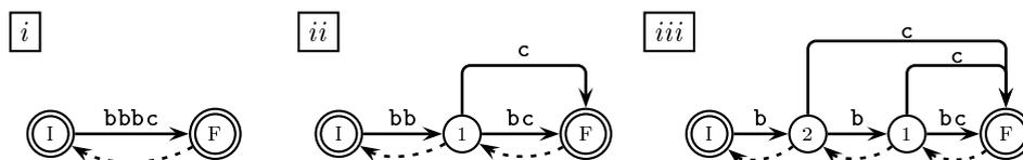
**Fig. 13.** Example of execution of *FastFind* ending with a solid edge during the construction of  $CDAWG(\text{bbbc})$ . The insertion of  $\text{suf}_1 = \text{bbc}$  leads to create state 1. Then *FastFind* works from I with path b. This leads to the middle of the edge (I,bb,1) (ii) that is solid. Since we cannot redirect this edge, state 2 is created, splitting (I,bb,1) into (I,b,2) and (2,b,1) (iii). The edge (2,c,F) is added,  $s_x(1)$  is set to 2, and  $s_x(2)$  is set to I.
