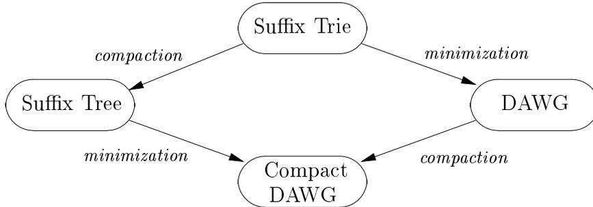
**Fig. 2.** Consider a word that has an end-marker. Its suffix tree is the compact version of the digital trie of its suffixes. Its DAWG is the minimized (in the sense of automata theory) version of the trie. The compact DAWG can be obtained either by minimizing the suffix tree of the word or by compacting its DAWG.
