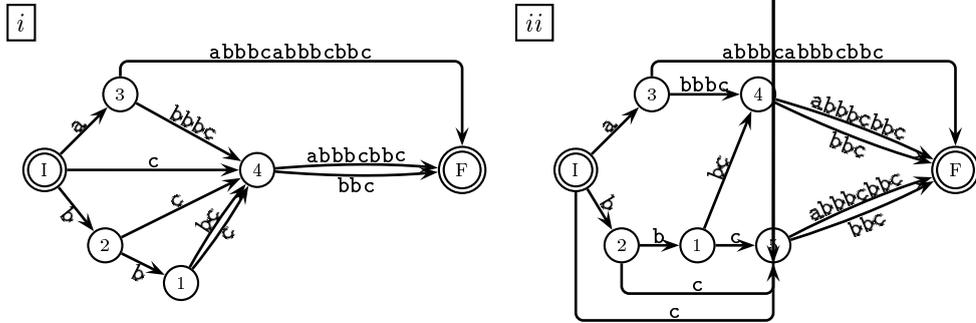
**Fig. 11.** Example of a duplication in *SlowFind* during the construction of  $CDAWG(aabbbcabbbcbbc)$ . The insertion of  $su_{f_1} = bbc$  leads to state 4. As the last edge  $(1,c,4)$  is non-solid (i), state 4 is cloned into state 5 (ii), and the edge  $(1,c,4)$  becomes  $(1,c,5)$ .
