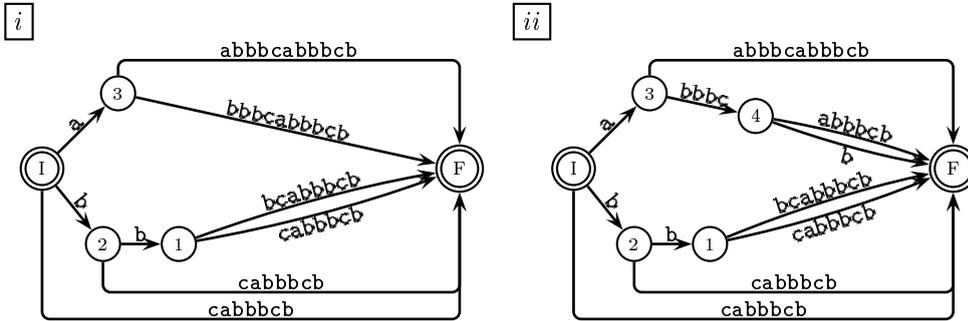
**Fig. 10.** Example of the execution of *SlowFind* during the construction of  $CDAWG(aabbbcabbbcb)$ . For the insertion of  $suf_6=abbbcb$ , we have  $head_6=abbbc$ . Since the path labeled by  $abbbc$  ends in the middle of the edge  $(3,bbbcabbbcb,F)$ , state 4 is created, splitting the edge into  $(3,bbbc,4)$  and  $(4,abbbcb,F)$ . A new edge is created,  $(4,b,F)$ .
