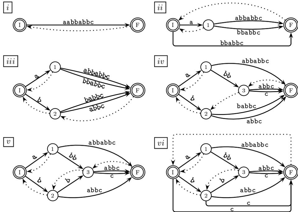
**Fig. 8.** Six steps during the construction of  $CDAG(aabbabbc)$ . The pictures display the situation after the insertion of  $suf_0 = aabbabbc$  (i),  $suf_2 = bbabbc$  (ii),  $suf_3 = babbc$  (iii),  $suf_4 = abbc$  (iv), and  $suf_5 = bbc$  (v). *vi* shows the final automaton.
