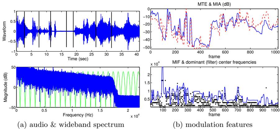
**Fig. 1.2.** Feature extraction from multi-source audio stream. (a) Waveform with manual labeling of the various sources/events (vertical lines) and wideband spectrum with filterbank, (b) top: MTE (solid) and MIA (dashed), bottom: MIF with dominant carrier frequencies superimposed (1024 frames from “300” video).
