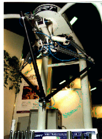
Figure 4. Speed-R-Man, a kinematically redundant PKM.
