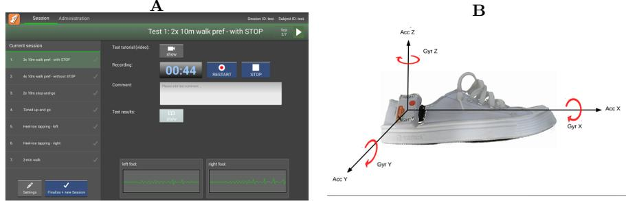
Fig. 1: Interface eGaiT and shoe with its attached inertial sensor.
