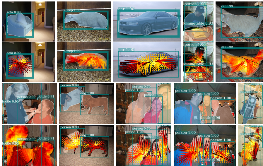
Fig. 5. Instance segmentation on Pascal VOC 2012. Each pair of rows visualizes instance segmentations produced with method, together with the corresponding semi-convolutional embeddings
