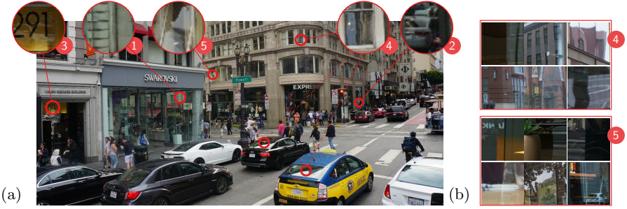
Fig. 2: Depending on the ratio between transmitted and reflected radiance, a semi-reflector may produce no reflections ①, pure reflections ②, or a mix of the two, which can vary smoothly ③, or abruptly ⑤. The local curvature of the surface can also affect the appearance of the reflection ④. The last two, ④ and ⑤, are all but uncommon, as shown in (b).
