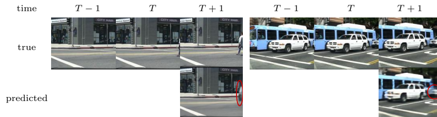
Fig. 2: Examples of failed prediction for car-cam video sequences. The first rows are the true frames and the second rows are predictions. T-1 and T are the last two input frames, and T+1 is the current output frame. As can be seen in the predicted frame at time T+1 , some details of objects which did not appear in the last frames, are missed.
