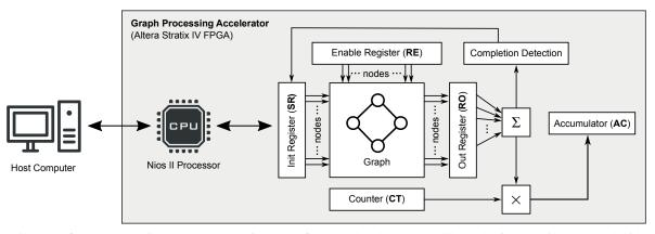
Fig. 4: Architecture of graph processing accelerator. An instance of the graph to be processed is synthesised and implemented with additional control circuitry and an on-board NIOS II processor. Host computer communicates with the accelerator via a JTAG interface and can initiate or read computation results using an Application Programming Interface (API) for graph processing.
