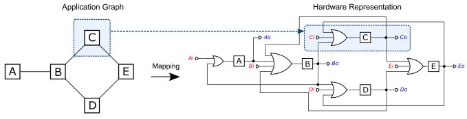
Fig. 5: Mapping a graph to a digital circuit for implementing on an FPGA.
