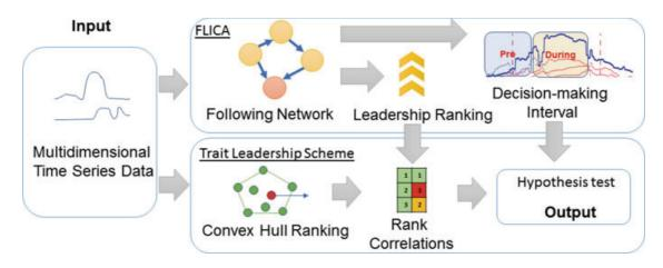
**Fig. 2** High-level overview of trait leadership scheme using FLICA ([1, Figure 1] used and modified with permission). An arrow between elements represents a relationship that an element at the rear of the arrow is the input of an element at the head of the arrow. For example, rank correlations are calculated by taking leadership ranking and convex hull ranking as inputs
