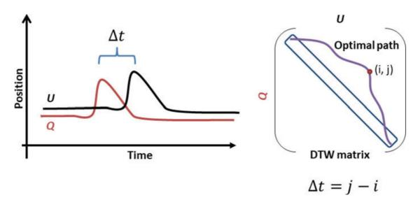
Fig. 3 An example of a following relation between time series U and Q. (Left) Time series U follows Q. (Right) The optimal warping path on the DTW dynamic programming matrix, shifting U backward in time onto Q
