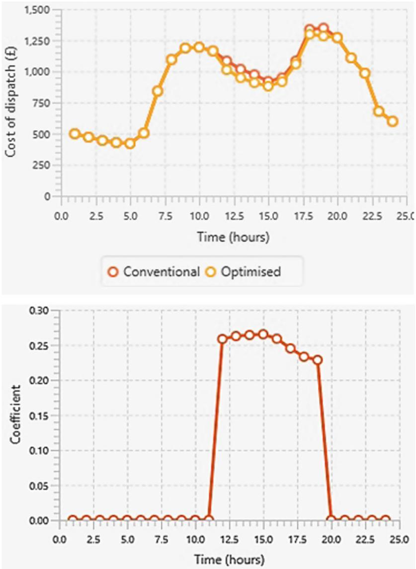
**Fig. 2.** Resilience coefficient and monetary costs calculated for the grid: top panel – plot of monetary savings in relation to the business-as-usual and the optimized solution; bottom panel – the distribution of resilience coefficient. Outage starts at 1200 with durations of eight hours.
