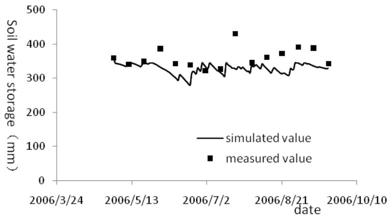
**Fig.3.** Comparison Chart of measured and simulated values of soil water storage with irrigation
