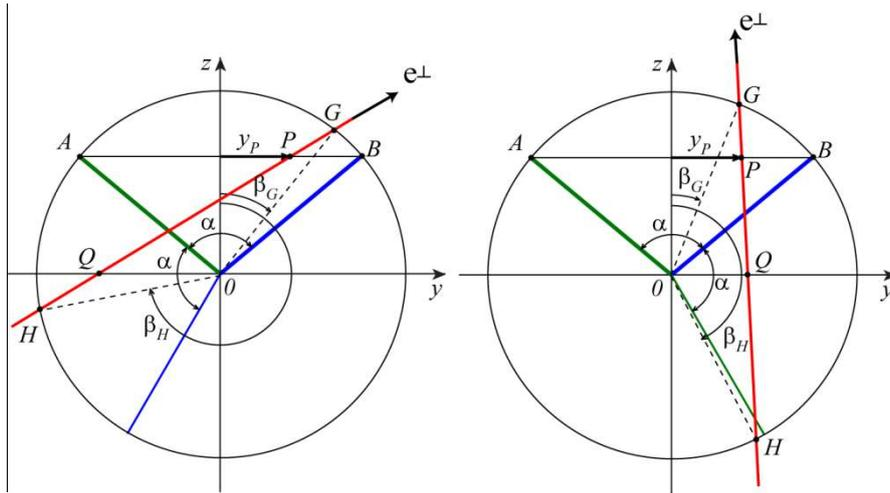
Figure 4 – Geometry for the calculation of the number of reflections, for a same position  $y_p$  of the ray, and two different orientations.
