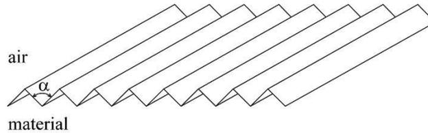
Figure 1 – Structured surface with parallel and periodical V-shaped ridges of aperture angle  $\alpha$ .
