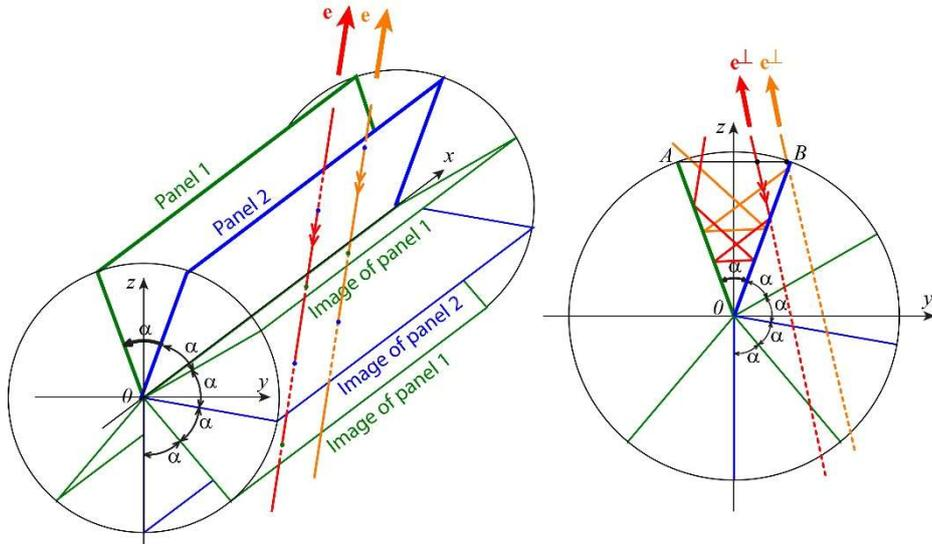
Figure 3 – Left: 3D representation of two parallel light rays oriented according to a same vector  $\mathbf{e}$  striking the cavity in different positions on panel 2. Right: 2D representation of the two same light rays projected onto the  $(yOz)$  vertical plane. The light path can be represented by a straight line meeting the successive images of the panels from each other. The projection of real light paths in broken straight lines is also represented on the figure (left).
