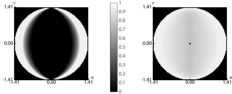
Figure 6 - Maps of angular reflectance for a  $45^\circ$  V-cavity made of silver, at 550 nm ( $n = 0.1249 + i3.3391$ ), represented with the Lambert azimuthal equal area projection, where only one reflection (left) and all the possible reflections (right) of rays in the cavity are rendered.
