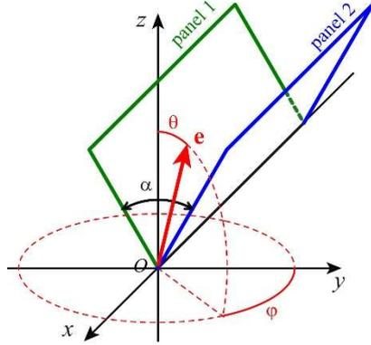
Figure 2 – 3D geometry of one cavity, and vector  $\mathbf{e}$  representing the direction of illumination.
