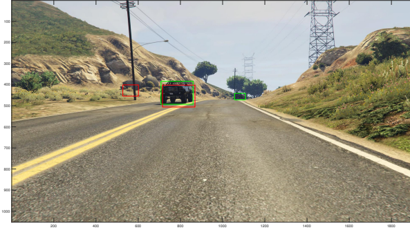
Fig. 4. GTA frame with red bounding boxes around cars detected by YOLO, and green boxes around true cars. Note the red box around the bush on the left, indicating a YOLO false positive, and the lack of red box around the faraway car on the right, indicating a YOLO false negative. The red box in the middle is a true positive.
