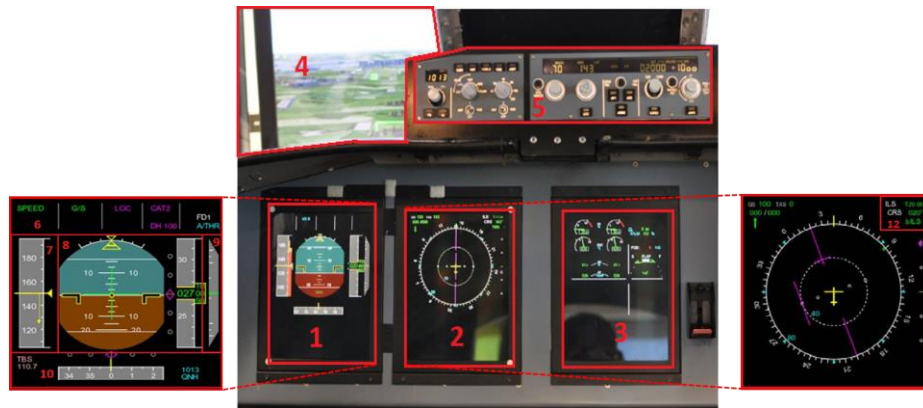
Fig. 3. Cockpit Display with AOIs and Sub-AOIs: (1) Primary Flight Display (PFD), (2) Navigation Display (ND), (3) Electronic Centralized Aircraft Monitoring (ECAM), (4) Out of Window (OTW), (5) Flight Control Unit (FCU), (6) Flight Mode Annunciator (PFD.FMA), (7) Speed Tape (PFD.SPD), (8) Attitude Indicator (PFD.ATT), (9) Vertical Speed Tape (PFD.VS), (10) Heading Tape (PFD.HDG), (11) VOR tag reading area in ND (ND-zone).
