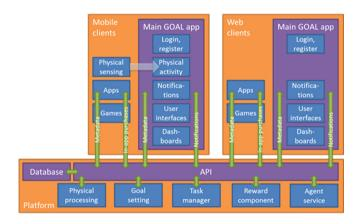
Fig. 1. High-level GOAL modular platform architecture.
