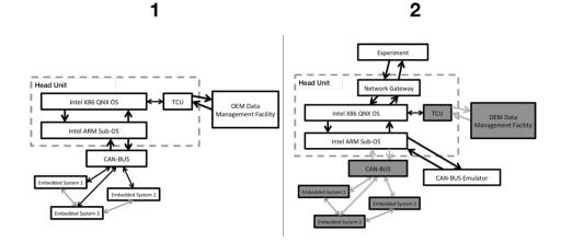
Fig. 1. The architecture as understood at a high-level is shown on the left-hand side. The right-hand side highlights the entry-method that was used. The sections of the original system that needed to be bypassed have been greyed out.
