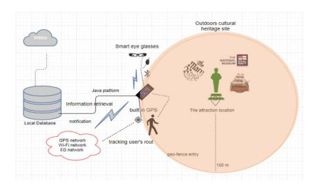
Fig. 1. Architecture of SmartC
