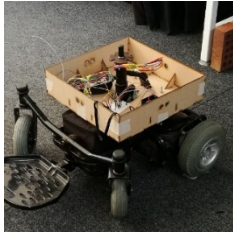
Fig. 2(a). The autonomous vehicle modified from the mobility scooter
