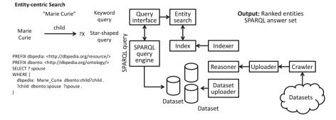
Fig. 7.3 High-level architecture components for Sindice (entity-centric search) [111]
