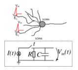
Fig. 1: Equivalent electronic circuit of the leaky-integrate-and-fire neuron model. Let a current I(t) charge the *RC* circuit. Spikes are generated when the voltage  $V_m(t)$  at the terminals of the capacitance is greater or equal to the threshold  $V_{th}$  making  $V_m(t)$ dropping to  $E_L$  (reset voltage) during a  $t_{ref}$  (refractory period).
