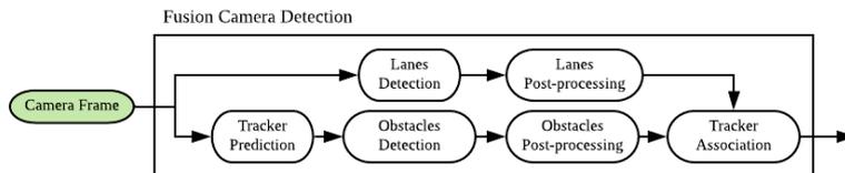
Fig. 3: Obstacle Camera Pipeline
