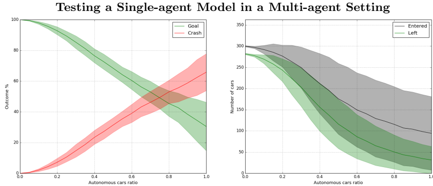
Fig. 4: Performance of the single agent model in a multi-agent setting with various ratios of autonomous cars present on the highway. The drop in performance is a clear indication for the need of a model trained in a multi-agent setting, that allows the policy to also incorporate a response to the behaviour of other autonomous agents.
