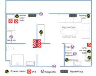
Fig. 1. Sensors system installed in the field trial apartment.
