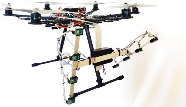
**Fig. 4.** Positioning system integrated in a hexarotor platform.
