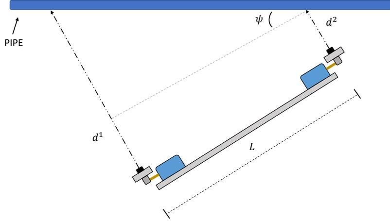
**Fig. 7.** Estimation of the orientation (yaw angle) of the positioning system relative to a pipe from the distance measured by both arrays.
