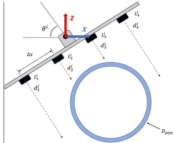
**Fig. 3.** Geometric model of an array of sensors tracking the contour of a pipe.
