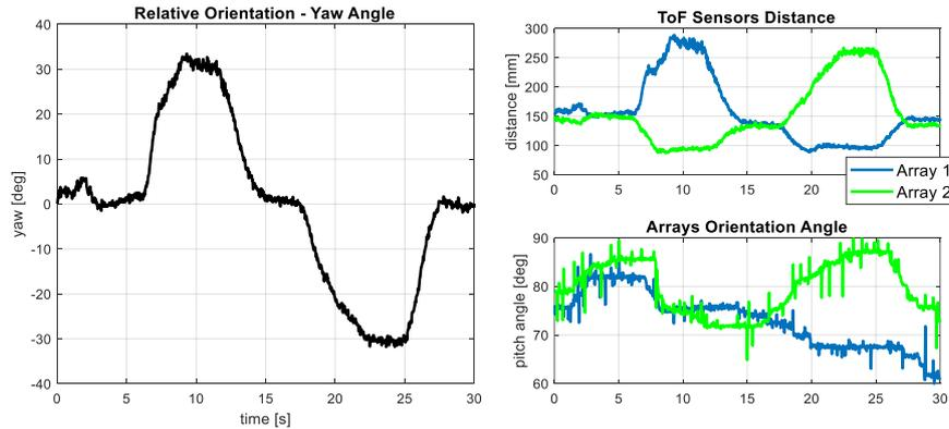
**Fig. 12.** Estimation of the relative orientation of the pipe in the yaw angle.
