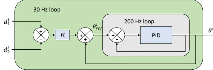
**Fig. 6.** Low level controller of the positioning system used in the tracking mode: inner PID position control loop and outer proportional controller used for aligning the internal sensors.
