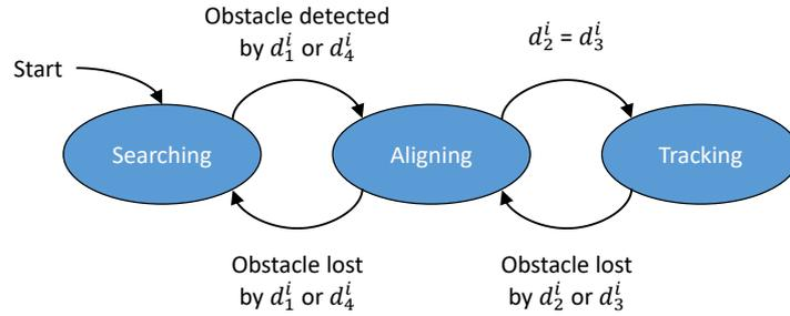
**Fig. 5.** State machine representing the three operation modes and transitions of the system.
