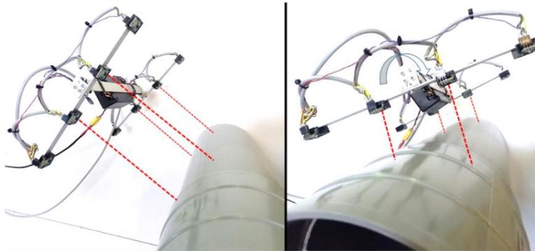
**Fig. 11.** Two poses of the positioning system while tracking the contour of the pipe.
