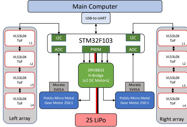
**Fig. 2.** Hardware architecture and components of the positioning system.
