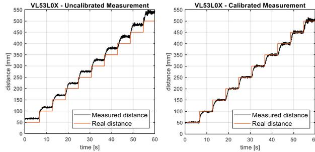
**Fig. 8.** Positioning accuracy of the VL53L0X-SATEL ToF sensor: uncalibrated (left) and calibrated (right) with offset correction. A 50 cm ruler is used as ground truth.
