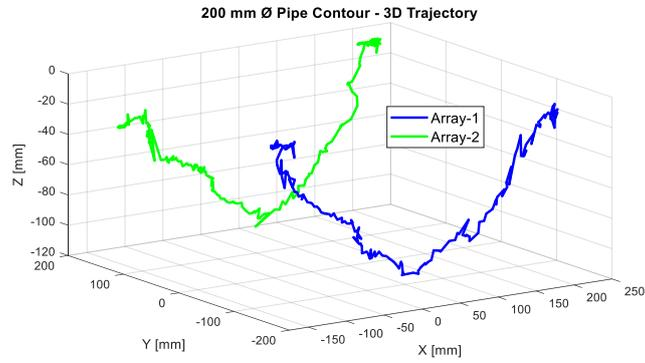
**Fig. 9.** 3D position estimation corresponding to the contour of the 200 mm Ø pipe.
