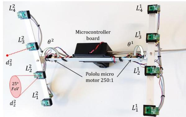
**Fig. 1.** Positioning system with two arrays of four time of flight sensors.
