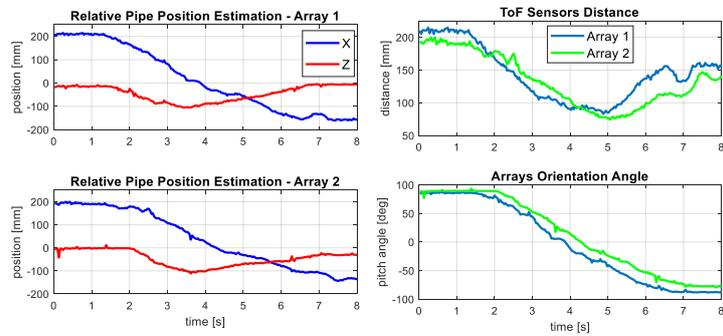
**Fig. 10.** Evolution of the relative position estimation provided by both arrays (left). Mean distance and orientation angle of the arrays (right).
