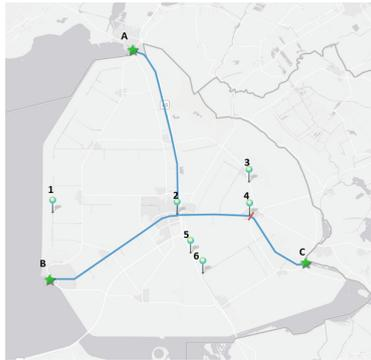
**Fig. 1.** Vital locations in the water management system of the Noordoostpolder. Numbers indicate water level measurement locations, letters indicate pumping stations. See Table 1 for a description of some of these points.
