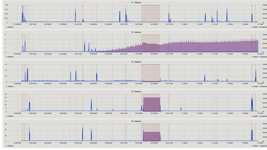
Fig. 2. Prediction errors for processes 1, 2, 3, 4, and 5 of SWaT (red: attack, purple: prediction error, and blue: anomaly score)
