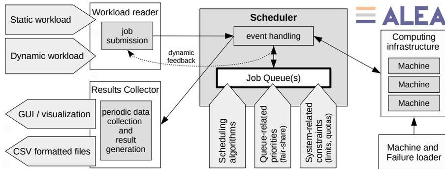
Fig. 1. Main parts of the Alea simulator.
