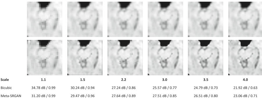
Fig. 8. (Top) Image going through various upsampling factors using Bicubic Interpolation. (Bottom) Image going through various upsampling factors using Meta-SRGAN. PSNR and SSIM scores are calculated against a target image downsampled by a factor of 4.
