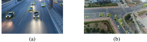
Fig. 4: (a) An example frame of UA-DETRAC and its ground-truth annotations. (b) An example frame of UAVDT and its ground-truth annotations.
