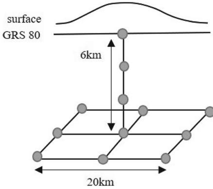
**Fig. 5.** Location of the input points. The magma distribution is interpolated with one-dimensional or two-dimensional linear functions, and input points represent control point of the magma distribution.
