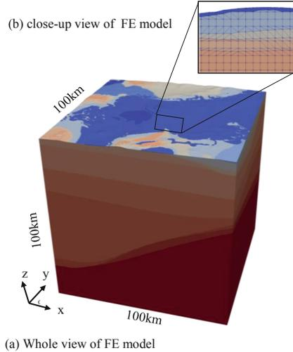
**Fig. 4.** Overview of the finite element model.
