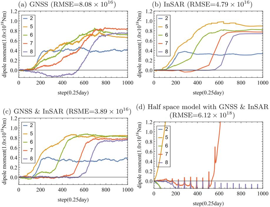
**Fig. 9.** Estimated strength of each dipole (Nm) with the observation data (a) GNSS alone (b) InSAR alone (c) GNSS & InSAR on the three-dimensional heterogeneous models. (d) is the result using Half space model with GNSS & InSAR. The numbers in the legend correspond to nodes shown in the Fig. 6. A result closer to the input trend in Fig. 8; a lower RMSE is preferable.
