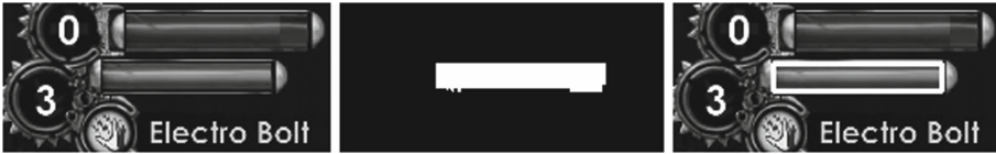
Fig. 3. Algorithm for detecting the value of the energy bar. From the left: The input area of the image detected by the classifier (additionally automatically cropped to improve processing); the image with detected pixels of proper shade and brightness (light blue); the output image with the outline of the energy bar marked, whose width is information about the energy possessed (fragments of processed frames from a screen-cast recorded from “Bioshock 2” [1]). (Color figure online)
