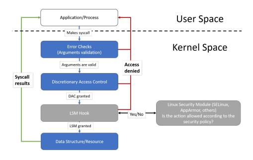
Fig. 4. Linux Security Modules (LSM) hooks.
