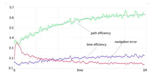
Figure 7. Progress of navigation path efficiency, navigation error fraction, and travelling time efficiency over learning time (simulation steps, with 200 vehicles, total occupied street capacity 10%, no pre-trained RL networks)
