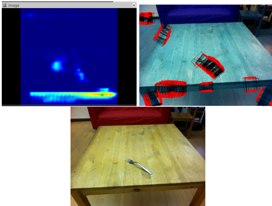
Figure 27: Grasp predictions by the two neural networks for a small object
