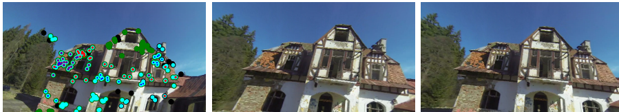
Fig. 1. Removing RS and radial distortion simultaneously using our minimal absolute pose solver. The original image (left) with tentative correspondences (black) the inliers captured by P4Pfr+R6P [4] (blue) and subsequent local optimization (red) compared to inliers captured by the proposed R7Pfr (cyan) and subsequent local optimization (green). The correction using R7Pfr without local optimization (right) is better than by P4Pfr+R6P with local optimization (middle).
