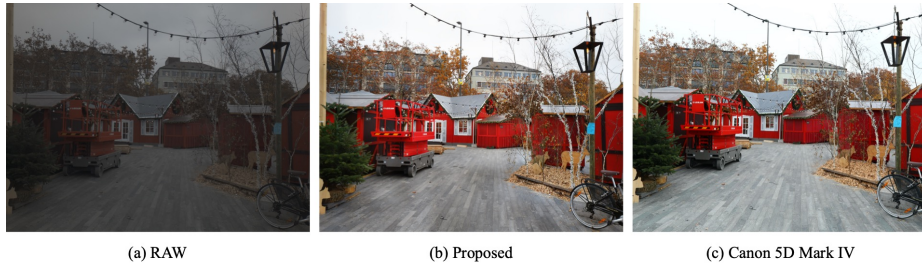
Fig. 1. Reconstructed RGB image from RAW data with the proposed method. (a) Input RAW image (visualised). (b) Reconstructed RGB image with proposed method. (c) Target image taken with Canon 5D Mark IV.
