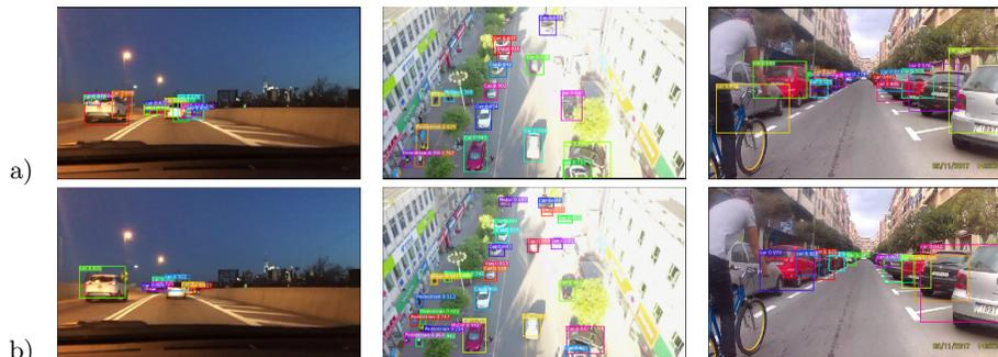
Fig. 4: Object detection results obtained from the application of the Mask R-CNN (a) and Flow R-CNN (b) models to the supported datasets[29, 30, 4]
