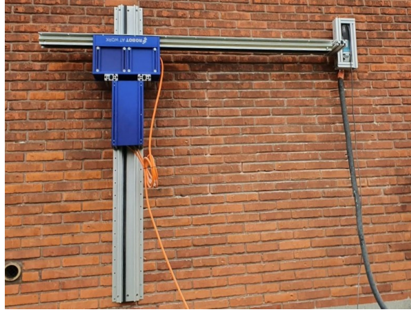
Fig. 1: An example setup of the autonomous mortar raking robot (designed by Robot At Work [18]). It is composed of a modular rail system to which electric motors are attached (blue housing in the image). The end tool is a milling device used to remove the mortar from between the bricks.
