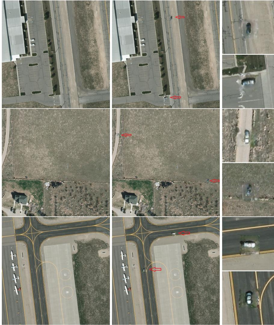
**Fig. 4.** Raw training images (left) are augmented with 2 separate car instances (middle). Augmented samples are highlighted with red arrows and their zoomed versions are shown on the right.
