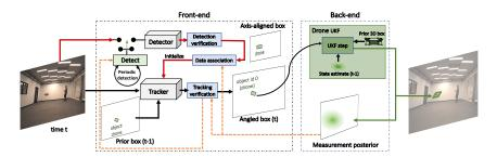
**Fig. 1.** Overview of MSL-RAPTOR. The front-end generates angled-bounding boxes & class labels from monocular images. The back-end tracks the object's pose with a class-specific UKF, and passes its uncertainty metrics to the front-end to detect when the tracker has lost the object.
